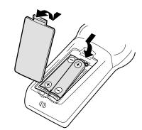
The batteries will last about six months with normal use If the functions of the remote control become erratic, replace the batteries
